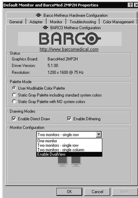
Figure 6: Barco Metheus Configuration Tab – Enabling DualView
