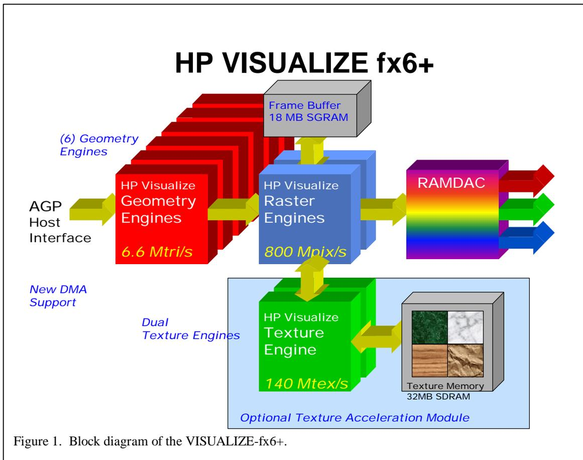
Figure 1. Block diagram of the VISUALIZE-fx6+.
