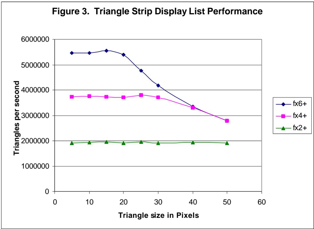
In application workloads that we have analyzed, most average triangle sizes are less than 25-pixels. While most data sets have large polygons as well, the small average size is due to approximating curved surfaces with a set of triangles.
