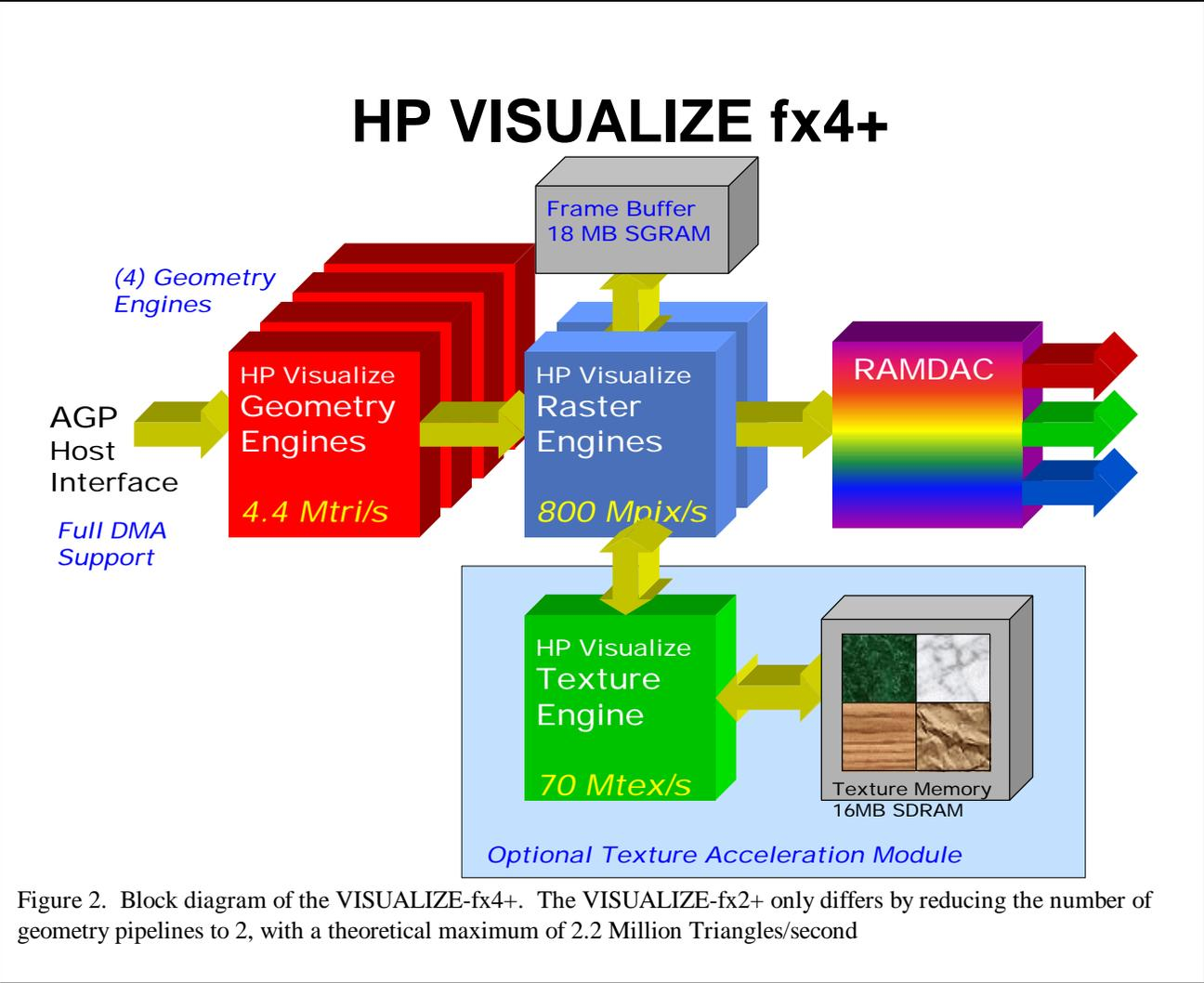
Although a similar naming convention is used, the VISUALIZE graphics products for the Windows NT environment are different implementations than for the Unix Workstation systems. The underlying architecture is the same. In particular, the Host Interface chip and the Rasterization chips are different in the Personal Workstation systems than in the Unix Workstation systems. In addition, the Windows products include VGA graphics for Windows compatibility when booting and for full-screen DOS mode.
