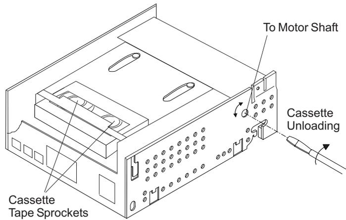
4. Insert a 1.5 mm hexagonal key or small Phillips screwdriver into the aperture on the right side of the drive near the rear. This gives you access to the motor worm wheel. Turn the hexagonal key or small Phillips screwdriver counter clockwise to release the cartridge (this action can take many turns of the screwdriver).
