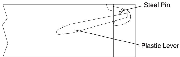
**Attention:** When attaching the bezel, the cassette door must be raised to make sure that the steel pin on the left side of the door (with the drive assembly facing you) is above the white plastic lever on the left side of the drive assembly.
