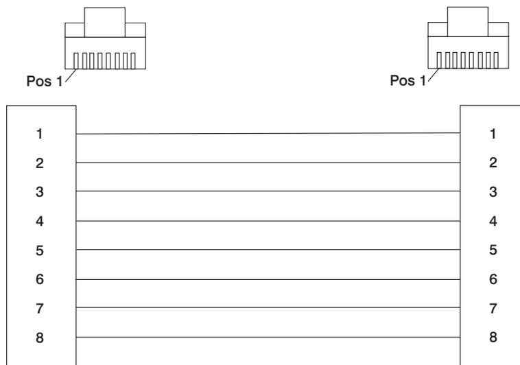
This cable is to be constructed using CAT-5 twisted-pair bulk cable (TIA/EIA 568A is recommended). The pairs must be wired as shown in the following table (the colors may differ; ensure that pin connections are correct). For additional information, see Ethernet specification IEEE-802.3u.
