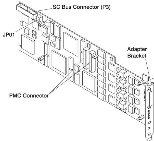
This IBM ARTIC960Hx 4-Port T1/E1 Mezzanine Card connects to the IBM ARTIC960Hx Base PCI Adapter by two 64-pin connectors. See “PMC Connector” on page 175. The interface signals exit the 4-Port T1/E1 Mezzanine Card through the 36-pin connector at the rear of the card. The IBM ARTIC960Hx Base PCI Adapter and the attached 4-Port T1/E1 Mezzanine Card occupy a single full-size 32-bit PCI expansion slot.
