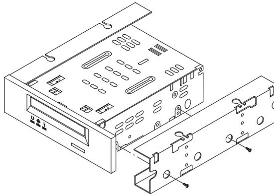
2. Remove the top cover by removing the four screws near the top edge of the tape drive (two on each side) and lifting the back of the cover.
