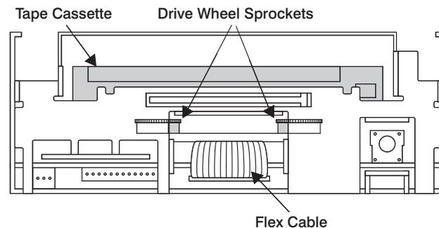
After the tape drive guidance rollers have fully retracted, turn the drive so that you are facing the front. With a small *non-magnetic* probe, access one of the drive reel sprockets and manually rotate the drive reels until all of the tape has been wound inside of the cartridge.
