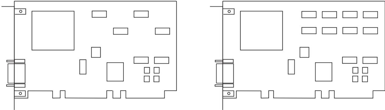
**Note:** In the illustration above, the GXT250P is on the left side and the GXT255P is on the right. The GXT255P has more modules in the upper-right quadrant of the adapter.
