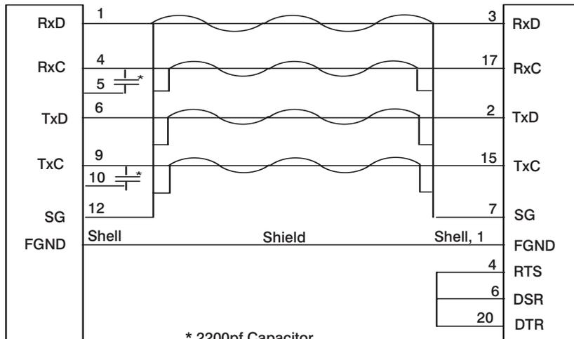
The 128-port async controller supports multiple controller line baud rates in EIA-232 synchronous-modem-attach mode. Although the 128-port async controller can operate at 57.6 Kbps, to ensure a low error rate on the synchronous link, controller line baud rates of 19.2 Kbps or less are recommended.
