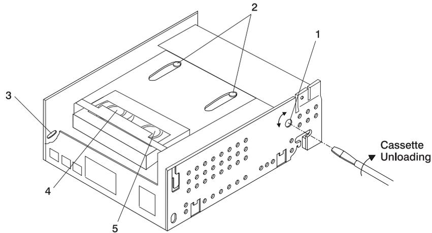
6. With a small flat-blade screwdriver, turn the mode motor gear inside the access hole, clockwise until the two pins **2** in the elongated slots begin to move toward the front of the drive (this action can take many turns of the screw driver).
