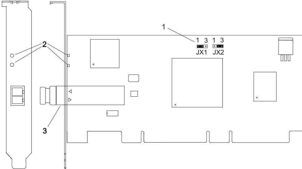
1. Jumper JX1, Pins 1 to 2 only and Jumper JX2, Pins 2 to 3 only
