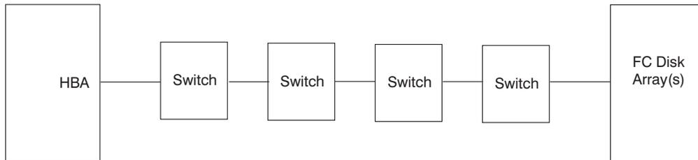
*Switches in a High Availability Configuration:* Due to its nature, Fibre Channel lends itself well to High Availability Cluster Multi-Processing (HACMP) environments. Switch configurations employing two or more host systems and two or more switches provide high availability capabilities so that in the event of failure of any one component, access to the data remains intact through an alternate path.
