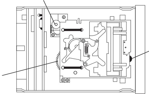
5. Push the front roller in and turn it clockwise until the tape is wound on the supply reel, and the roller stops.
