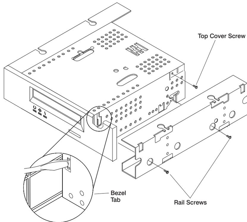
3. Remove the front bezel (the bezel snaps on).
