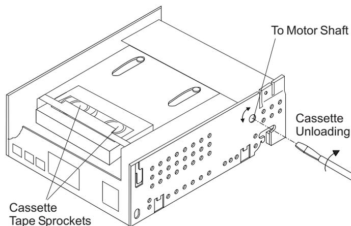
The following steps attempt to remove the tape from the drive without damaging the tape. In the following steps, it can take many turns of the screwdriver before the tape cartridge can be removed.
