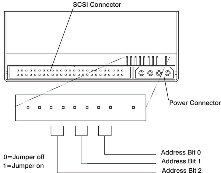
There are two pins for each bit. When a jumper is on (shorting two pins together) that represents a 1 in the following SCSI ID table. The three bits in the ID give a range of 0 through 7 as follows:
