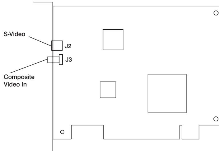
The Ultimedia Video Capture Adapter allows connection of the system unit to various video equipment.
