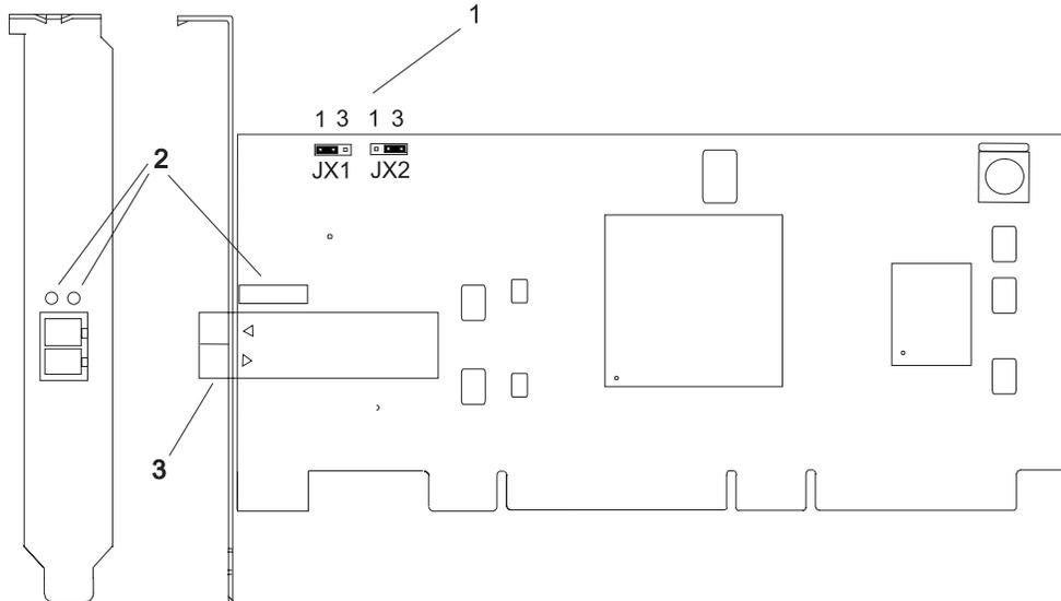
1. Jumper JX1, Pins 1 to 2 only and Jumper JX2, Pins 2 to 3 only
