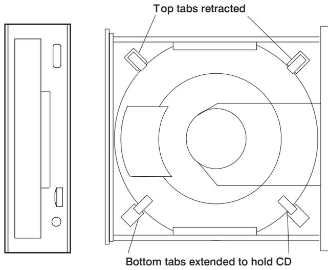
**Note:** All four tabs must be retracted when the drive is used horizontally.
