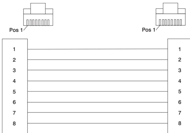
This cable is to be constructed using twisted-pair cable. The twisted-pairs of wires must be wired as shown in the following table. For additional information to construct your own cable, see Ethernet specification IEEE-802.3u. Ethernet cables must meet Ethernet specification IEEE-802.3u.
