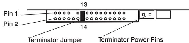
Disk drive types I1 and I2 do not support on-board termination. When you use these drive types in a Machine Type 7043 Model 140 system, you must have an in-line terminator between the last disk drive and the SCSI cable connector for that disk drive.
