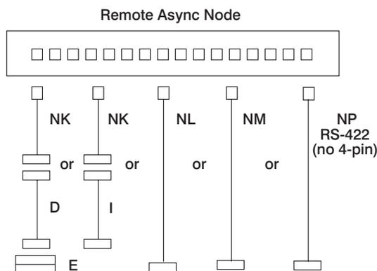
To make the necessary connections to the Remote Async Node, the system administrator must know the type of device that is being configured and its port location on the Remote Async Node. The cable planning charts section of the *Site and Hardware Planning Information*, order number SA38-0508 can help you make these assignments.
