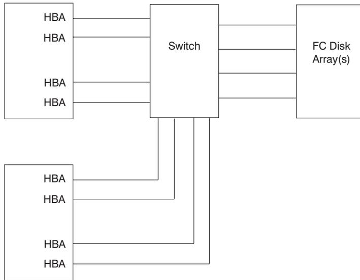
*Switch Configuration with Four Host Systems:* The following illustration shows an example of four host systems connected through a switch to a Fibre Channel disk array.
