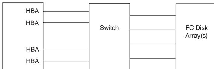
*Switch Configuration with Two Host Systems:* The following illustration shows an example of two host systems connected through a switch to a Fibre Channel disk array.
