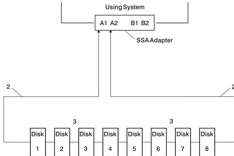
If a disk drive fails or is turned off, the loop is broken. At this point, one of the data paths to each disk drive is no longer available. The other disk drives continue to work through the remaining data path, but an error is reported to the system.
