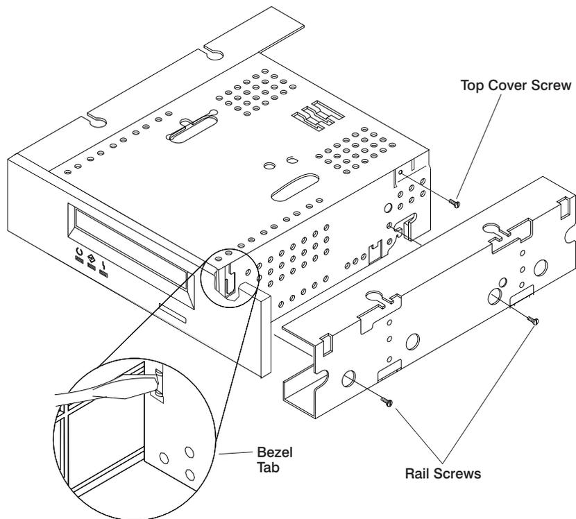
1. Remove the mounting rails by removing the four rail screws (two for each side).
