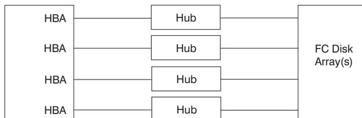
*Hub Configuration With Two Host Systems:* The following illustration shows an example of two host systems connected through hubs to a Fibre Channel disk array. In this example, each system is connected to both hubs.
