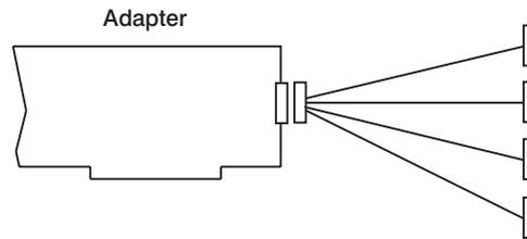
Each cable has a single 120-pin, male, D-shell connector that branches into four individual cables, each of which provides access to one of four independent ports.
