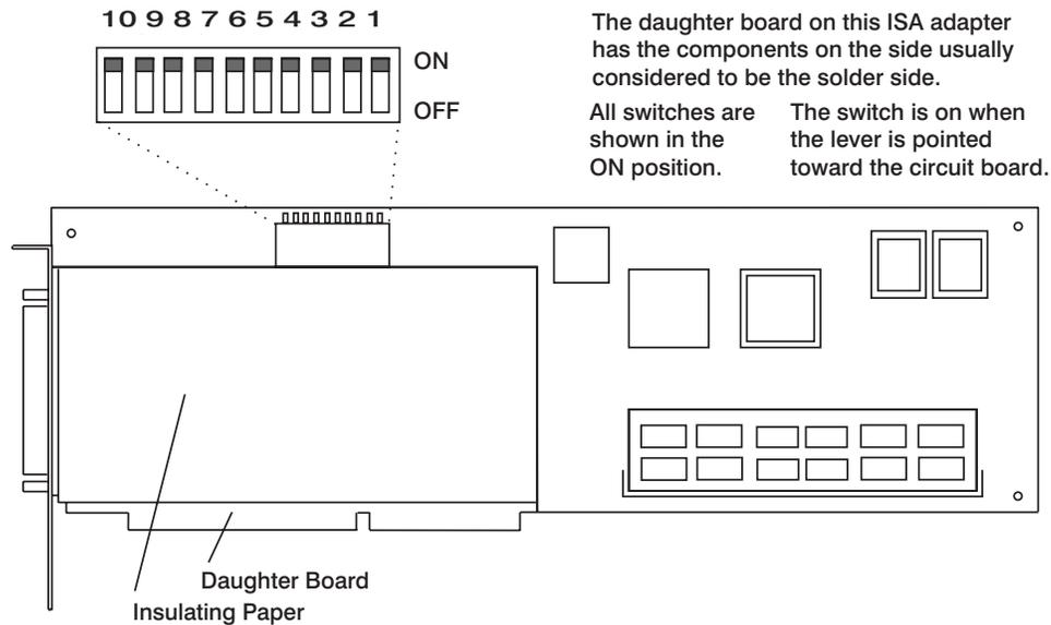
**Note:** The 10-pin switch on this adapter is labeled "Open" and "Closed". This publication uses "on" and "off" to indicate the state of the switch.
