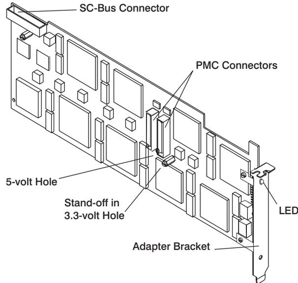
The IBM ARTIC960Hx DSP Resource PCI Adapter connects to the ARTIC960Hx Base Adapter by two 64-pin connectors. See “PMC Connector” on page 175. The interface signals exit the DSP Resource PCI Adapter through the 26-pin signal-computing bus (SC-bus) connector at the top of the PCI Adapter. The IBM ARTIC960Hx base adapter and the attached DSP Resource Adapter occupy a single full-size 32-bit PCI expansion slot.
