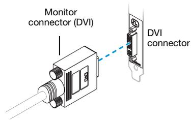
You can also connect an analog monitor with an HD-15 connector using an analog dual-monitor cable (included with certain Matrox products) or using a DVI-to-HD15 adapter. If you need this adapter and it's not included with your Matrox product, contact your computer vendor.
