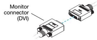
If you're connecting only one monitor, use the main connector (labeled **1** or **1/3**) of your dual-monitor cable.
