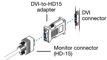
To use a dual-monitor cable to connect one or two analog monitors, connect it to your card and to your analog monitor cables. If you're connecting only one monitor, use the main connector (labeled **1** or **1/3**) of your dual-monitor cable.
