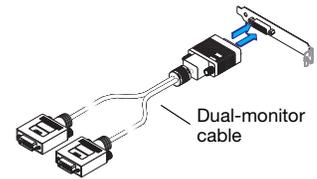
**Analog dual-monitor cable** – If you're using an *analog* dual-monitor cable (a cable with HD-15 connectors), you can only connect analog monitors. Connect your cable to your card and to your analog monitor cables. If you're connecting only one monitor, use the main connector (labeled **1** or **1/3**) of your dual-monitor cable.
