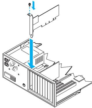
Your Matrox card is now installed. *Before restarting your computer*, connect your monitor or monitors (see “[Connection setup](#)”, page 6). *After connecting*, restart your computer and install your Matrox software (see “[Software installation](#)”, page 11).
