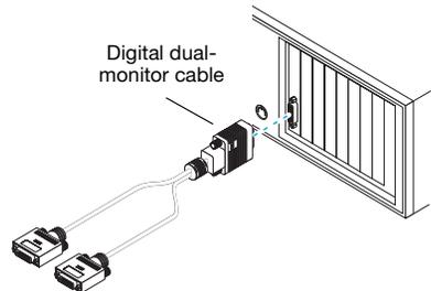
If your monitor has a DVI connector, connect it directly to the main DVI connector (**1/3**) of your dual-monitor cable.
